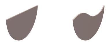
Figure 5: In-plane optimization. Example of the modification of the profile of an arbitrarily selected baffle. Initial flat-lined profile (left) and the outcome of the optimization (right).
