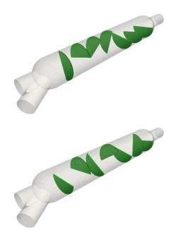
Figure 13: Positional Angle Optimization. Final positions of the baffles for the two extreme Pareto solutions. Top: positions when optimizing only for  $F_P$ ; bottom: positions when optimizing only for  $F_U$ .
