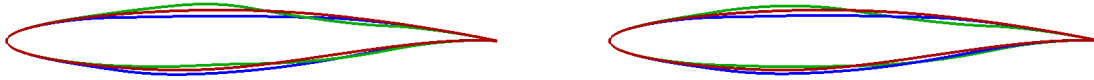
Figure 5: Comparison of the initial (red curve), \mu_F optimal (blue curve) and \sigma_F optimal (green curve) geometries designed by pFOSM (left) and iPCE (right).
