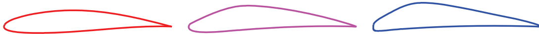
Figure 7: Optimization of a 2D isolated airfoil: Three airfoil shapes corresponding to the high lift-high drag part of the Pareto front (second sub-front) shown in fig. 5. From left to right the three airfoils yield the following C_L, C_D values: (0.968, 0.00978), (1.096, 0.010678) and (1.19, 0.01136).
