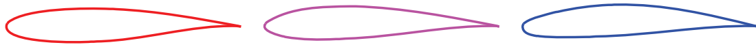
Figure 6: Optimization of a 2D isolated airfoil: Three airfoil shapes corresponding to the low lift-low drag part of the Pareto front (first sub-front) shown in fig. 5. From left to right the three airfoils yield the following C_L, C_D values: (0.707, 0.00901), (0.817, 0.00918) and (0.894, 0.00948).
