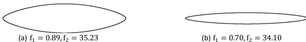
Figure 5: The initial (a) and the optimal (b) tube shape obtained by the one-shot optimization.
