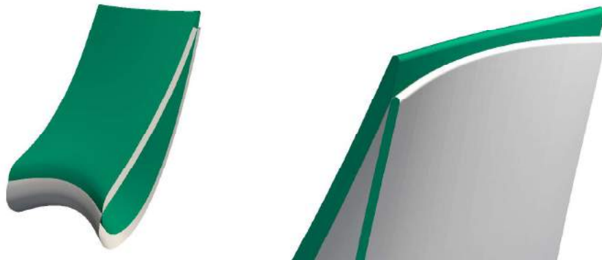
Figure 4.31: HPT stage. Objective function: axial force on rotor blade. Baseline (gray) compared to improved (green) stator blade geometry. Left: Pressure side. Right: Trailing edge close-up view.
