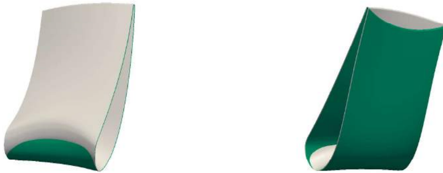
Figure 4.20: HPT vane. Baseline (gray) vs. improved (green) vane geometries. Left: Pressure side. Right: Suction side.
