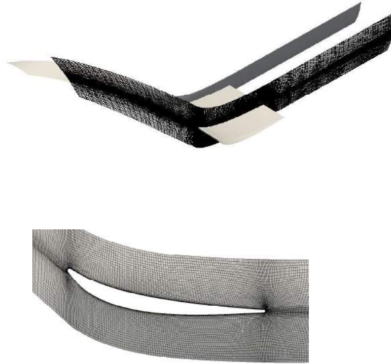
Figure 4.8: TurboLab stator. Geometry and radial grid cut at midspan.
