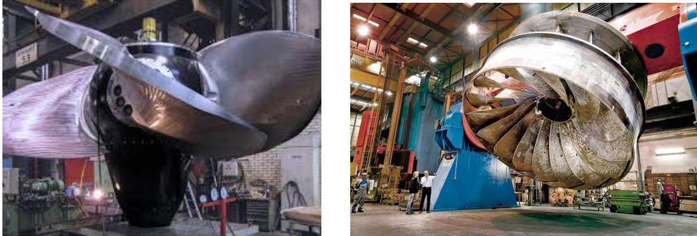
**Figure 1.3:** *Typical designs of Kaplan (left) and Francis (right) turbine runners. The specific models shown are designed by Andritz Hydro.*
