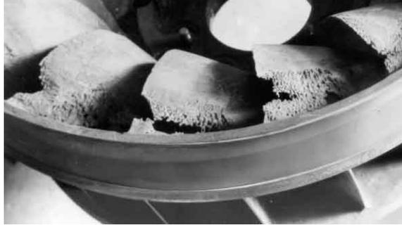
**Figure 5.6:** *The metal surface of a turbine's runner after extensive damage from cavitation [18].*
