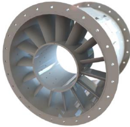
Figure 2.4: Assembly of the TU Berlin stator, from [16].
