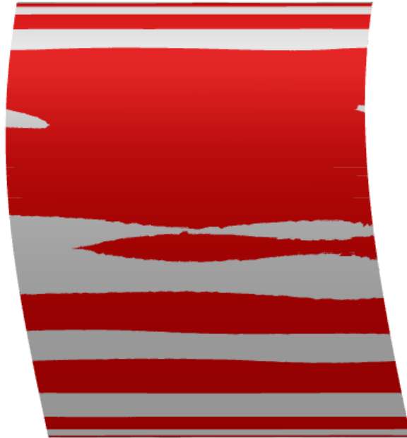
Figure 4.20: Initial (grey) and reparameterized (red) geometry of the TU Berlin stator plotted together, using N' = 5 generatrices in the reparameterization.
