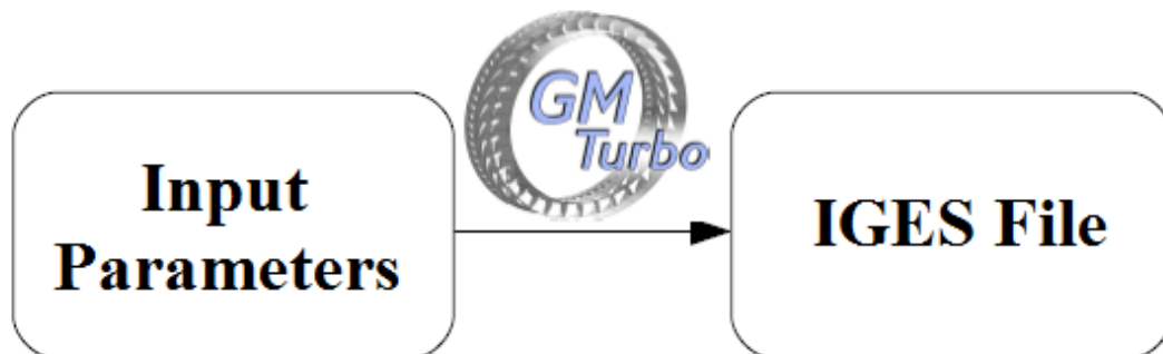
Figure 4.1: The GMTurbo generates the CAD compatible geometry of the blade.
