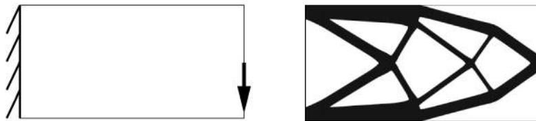
**Figure 2.1:** *The concept of TopO in structural optimization: Left: Computational domain and the applied loads and boundaries for the design of a cantilever beam. Right: Solution from TopO. White areas correspond to void (zero material density) whereas dark areas correspond to the designed structure (high material density). From [30].*
