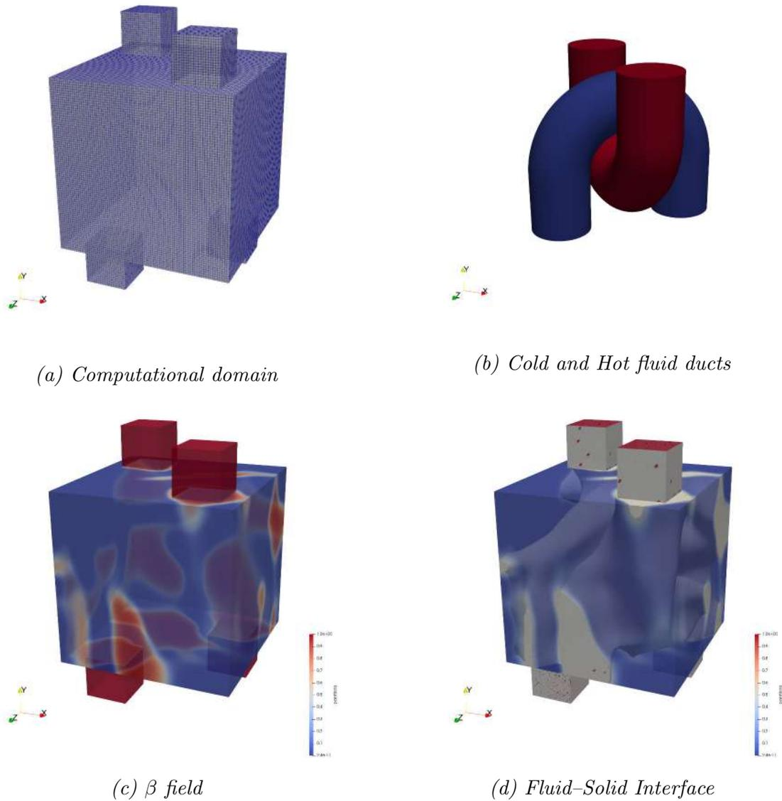
**Figure 5.22:** TopO of a Bi-Fluid 3D Heat Exchanger of 1 inlet and 1 outlet for each fluid. (a) Computational domain and (b) initial geometry of cold (blue) and hot (red) fluid ducts. (c) The  $\beta$  field computed from porosity-based TopO and (d) the extracted FSI geometry using the proposed algorithm.
