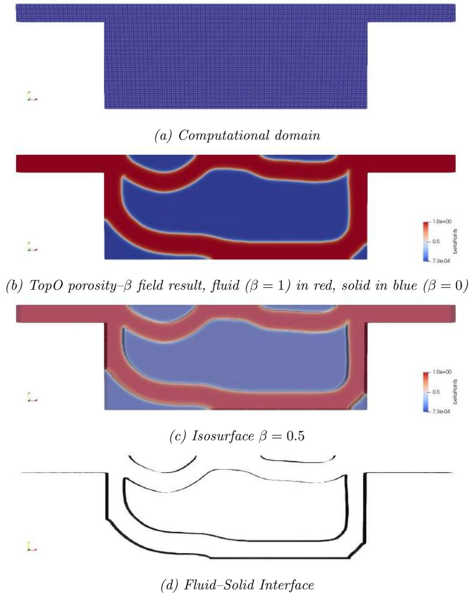
**Figure 5.21:** TopO of a 2D Heat Exchanger of 1 Inlet and 1 outlet. (a) Computational domain, (b) the  $\beta$  field computed from porosity-based TopO, (c) the Isosurface  $\beta = 0.5$  under consideration and (d) the extracted FSI geometry using the proposed algorithm.
