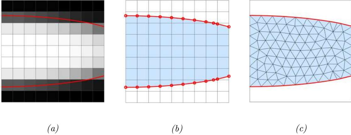
**Figure 2.3:** *Fluid nozzle illustrating the basic differences among design representations in topology optimisation: (a) Standard Porosity-based representation (b) level set cut-cells representation (c) explicit boundary representation (body fitted mesh). Reproduced from [19].*
