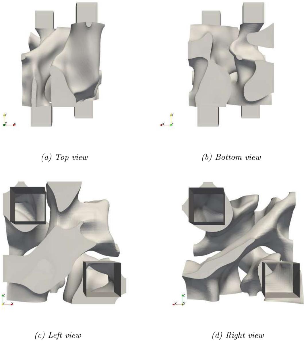
**Figure 5.23:** Views of the extracted FSI of the ducts of the two fluids for the heat exchanger. (a) Top, (b) bottom, (c) left, (d) right view.
