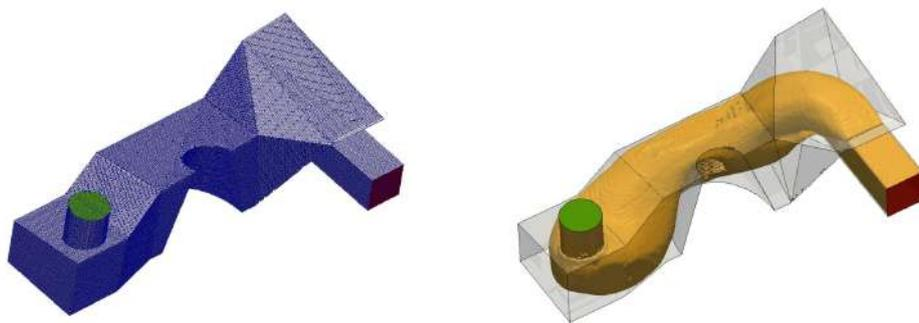
**Figure 2.2:** *The concept of topology optimization in fluid mechanics: Left: Computational domain for the design of an HVAC duct. Fluid flow from the inlet (green) to the outlet (red) subjected to performance objectives (e.g. minimum pressure losses). Right: Solution from topology optimization. Yellow area corresponds to the Fluid-Solid Interface. From [8].*
