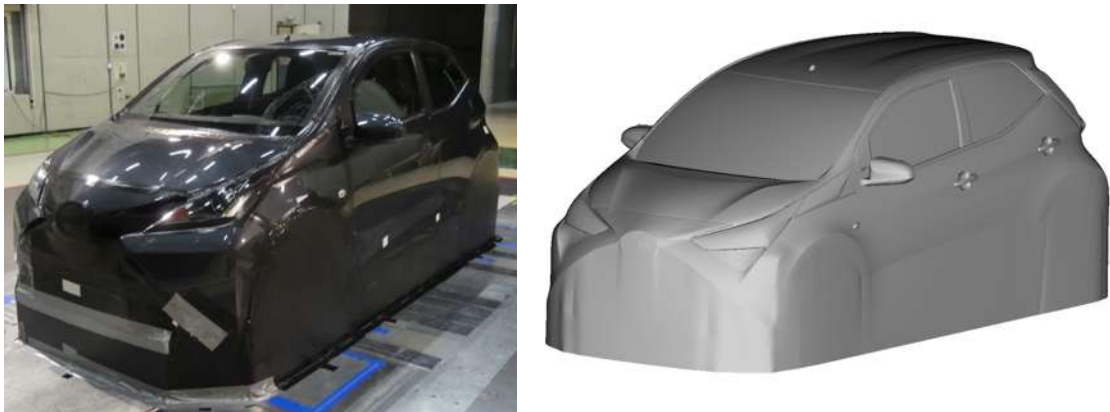
Figure 4.24: Application to a Production Car. A view of the actual car on the wind tunnel (left) and the simulated geometry (right).
