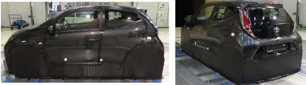
Figure 4.27: Application to a Production Car. Two views of the car with the skirt used to completely seal the underbody in the wind tunnel.
