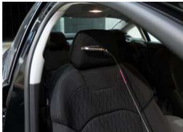
Figure A.4: A view of the microphone position in the interior of the car, close to driver's left ear. From [35].
