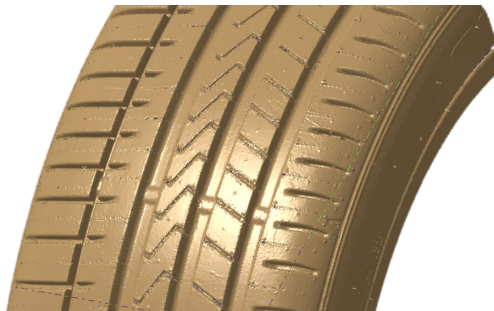
Figure 4.19: Point-Cloud of the 3D-Scanned tire.
