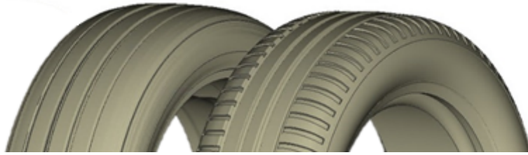
Figure 4.16: Grooved Tire geometry (left) and fully treaded tire geometry (right).
