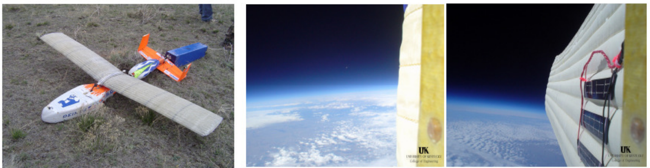
Figure 1.10: Big Blue Project, BIG BLUE II aircraft and attached inflation system at the recovery site (left). BIG BLUE 3 pre-inflated (middle) and post-inflated (right) at maximum altitude.
