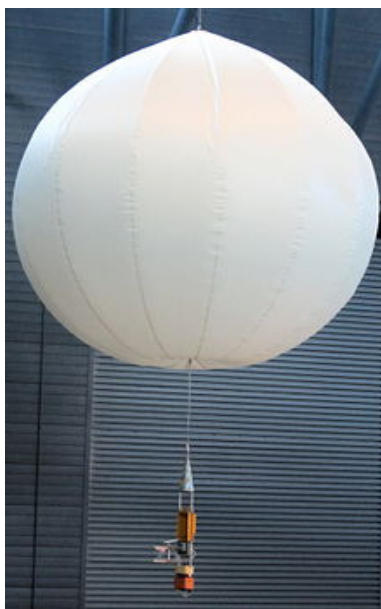
Figure 1.4: Replica of the balloon used in Venus exploration, [10]
