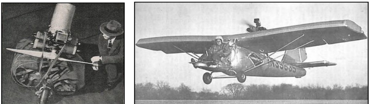
Figure 1.7: Goodyear's Inflatoplane. Left: The inflatoplane in the deflated state. Right: The inflatoplane during test flight. [11]
