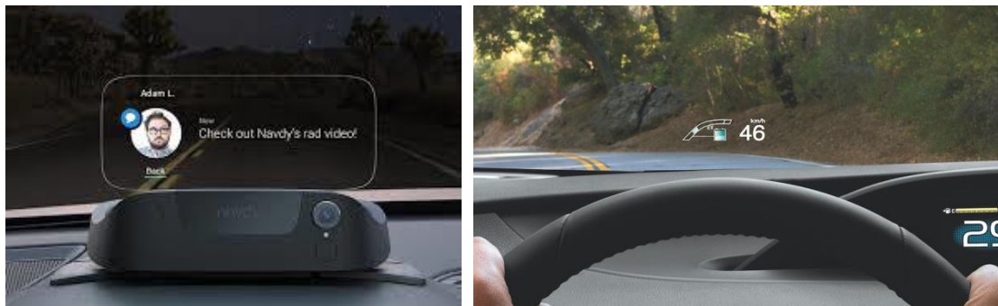
Figure 5.1: Examples of On-board (left) and In-Car (right) Head-Up Displays
