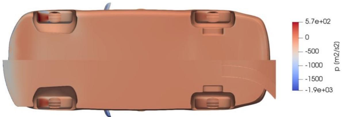
Figure 4.9: Comparison of the pressure distribution on the car body, between the original car geometry (top) and the modified geometry (bottom), in bottom view. The colour scale is the same for the two fields and the zero is set to the ambient pressure.
