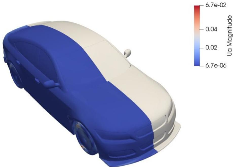
*Figure 5.4: Adjoint velocity magnitude distribution on the modified car body, in front 3/4 high elevation view. Results are presented on the right half of the car.*
