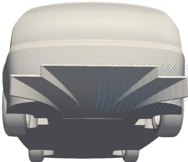
*Figure 6.2: The movable control points for the rear diffuser. Some control points are located inside the car geometry and they are not visible.*
