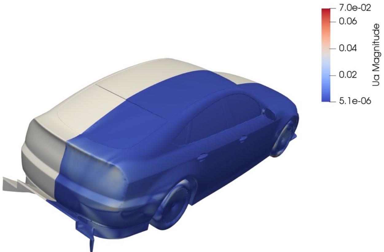
Figure 5.6: Adjoint velocity magnitude distribution on the modified car body, in rear 3/4 high elevation view. Results are presented on the right half of the car.
