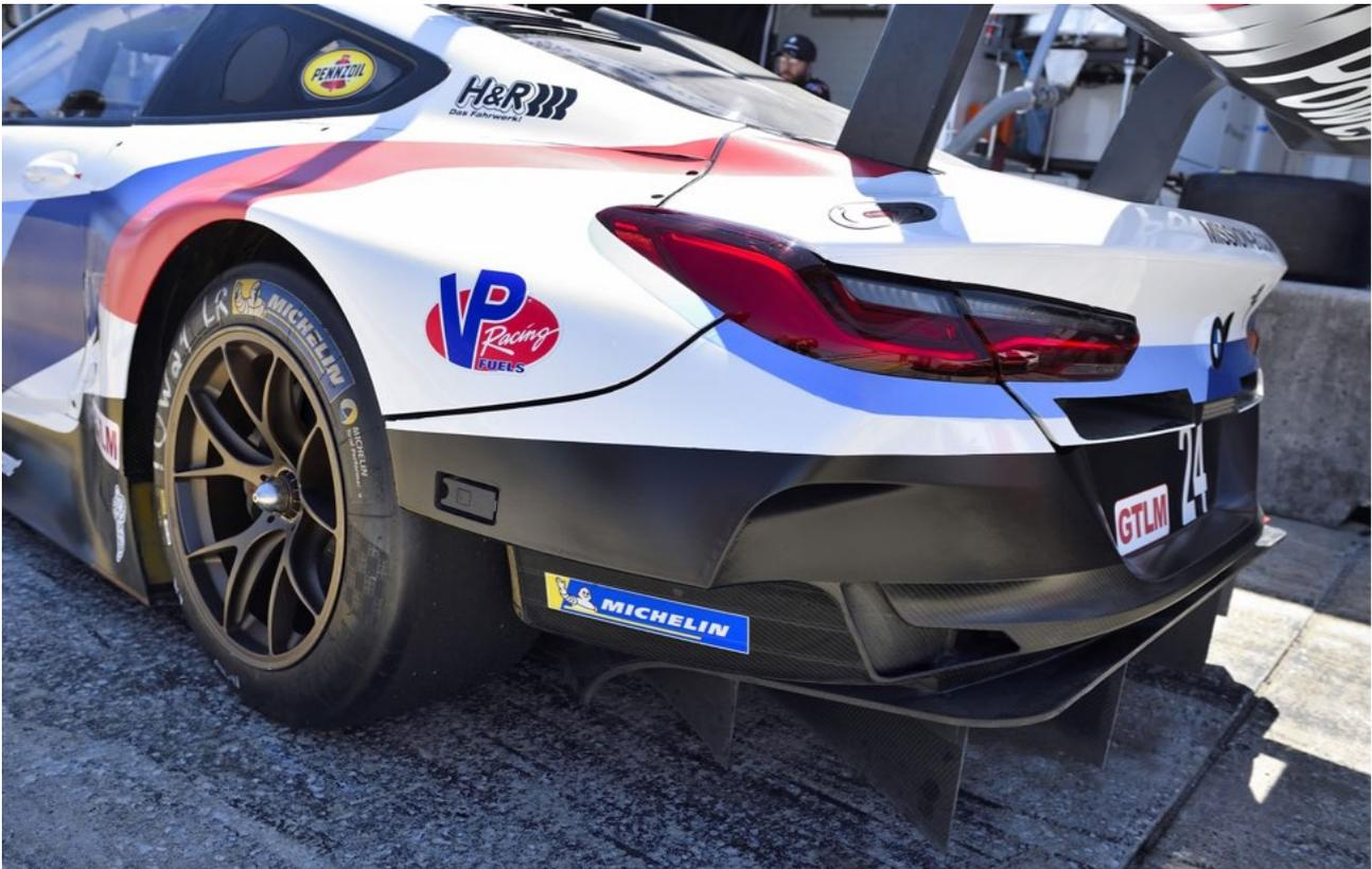
Figure 2.10: Top to bottom: Different solutions for the rear diffuser. A rectangular diffuser on the Aston Martin Vantage<sup>21</sup>, a stepped rectangular diffuser on the Porsche 911 RSR<sup>22</sup> and a curved diffuser on the Ford GT<sup>23</sup>. The diffuser of the BMW M8 GTE<sup>24</sup>, which has open sidewalls is also shown at the very bottom.
