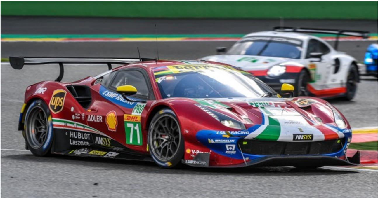
Figure 2.8: Different solutions for the front splitter. A flat splinter on the Chevrolet Corvette C7.R<sup>18</sup> (top) and a curved splitter on the Ferrari 488 GTE EVO<sup>19</sup> (bottom).
