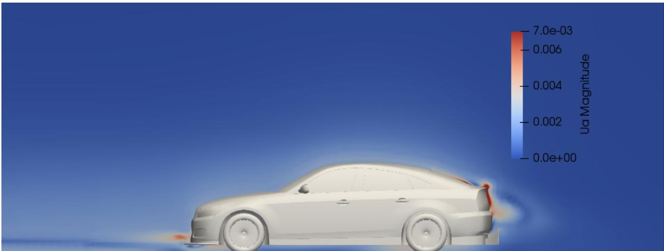
*Figure 5.3: Adjoint velocity magnitude at the modified car symmetry plane.*
