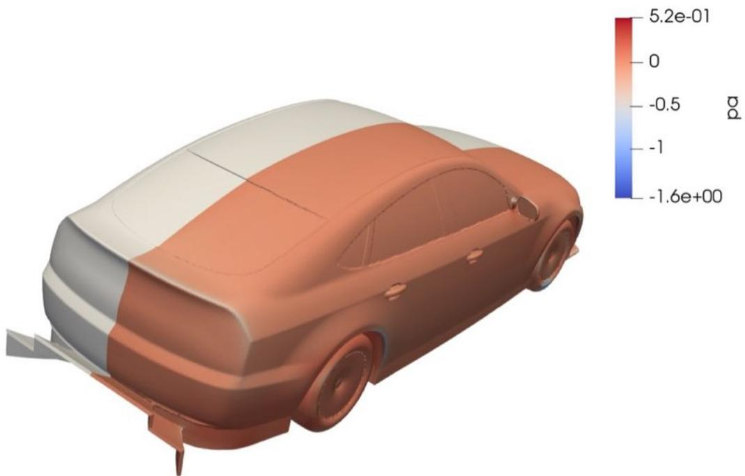
Figure 5.11: Adjoint pressure distribution on the modified car body, in rear 3/4 high elevation view. The results are presented on the right half of the car.
