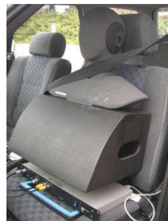
Figure 5.1: Binaural head model for noise level measurements in vehicle cabins. (Sourced from [55])
