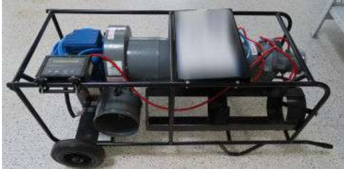
(a) Airflow Generator
