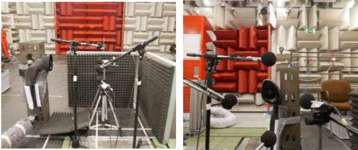
Figure 5.7: Microphone positions for blower noise measurement. Four microphones are used, marked as 0^\circ 90^\circ 180^\circ and 270^\circ .
