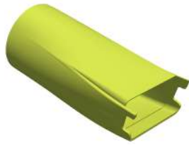
Figure 5.5: Adapter connecting the blower with the straight circular pipe. Left CAD model, right, 3D prototyped part.
