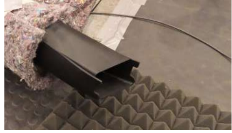
Figure 5.5: Adapter connecting the blower with the straight circular pipe. Left CAD model, right, 3D prototyped part.
