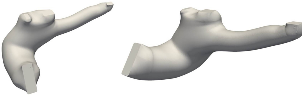
Figure 3.5: The duct after the smoothing the surface geometry topology optimization produced, fig. 3.4.
