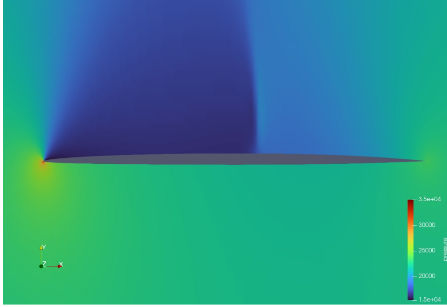
Figure 4.5: Pressure field around the n16103 airfoil.
