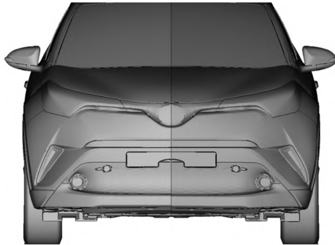
Figure 6.16: Optimized vs Baseline geometry - Front view - Optimized geometry on the right side of the figure.
