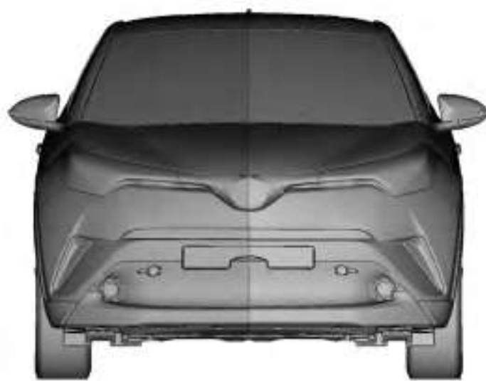
Figure 6.1: Baseline vs Optimized Front Bumper. Optimized geometry on the left side of the figure.
