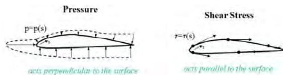
Figure 1.1: Pressure and stress distribution applied on a body immersed in a fluid. [22]
