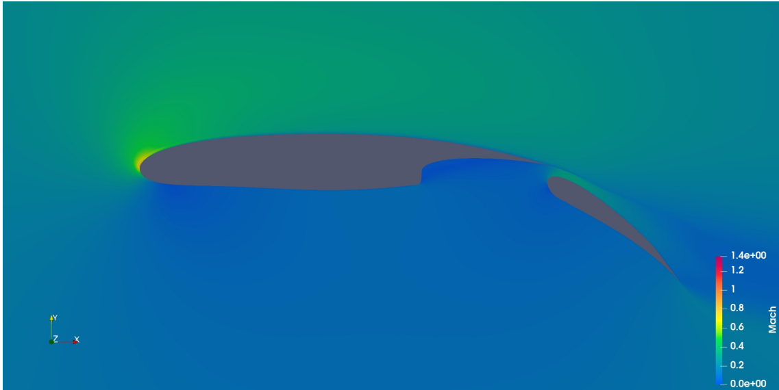
Figure 6.10: Case A3: Mach number field around optimized airfoil.
