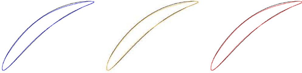
Figure 6.11: The compressor blade-airfoil case: The baseline (black) is compared to the optimized solutions obtained using adjoint (blue), DNN_A (orange), and DNN_B (red).
