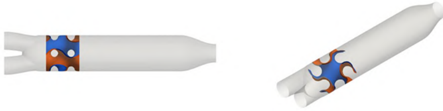
Figure 1.9: Static mixing device with a Gyroid geometry. Fluid enters from the left side and there is a common outlet on the right side, [16].
