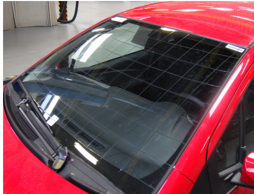
(a) Measurement grid from the outside.
