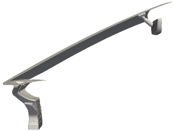
Figure 5.2: CAD data of the important parts of the model: defroster nozzle, instrument panel outlet, windshield, mirror.
