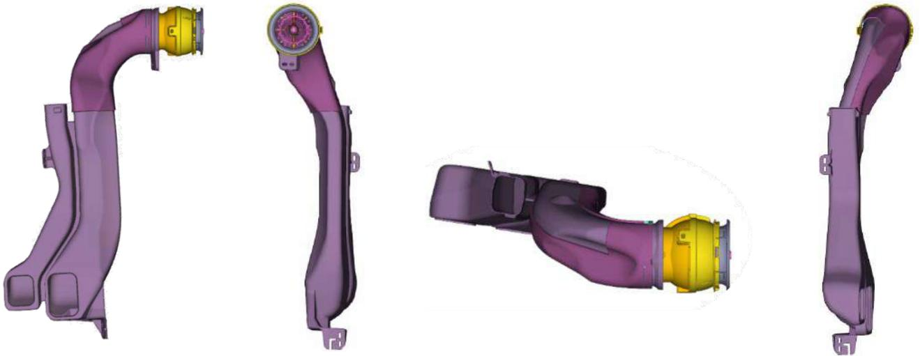
**Figure 6.2-3:** Side-duct assembly of car two.
