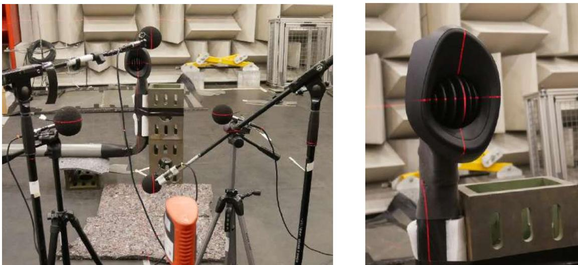
**Figure 6.3-2:** Alignment of test piece and microphones with the use of a laser cross.
