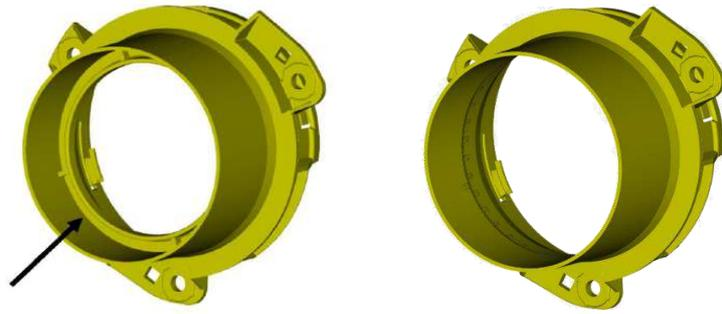
**Figure 6.2-2:** Original register's housing (left) versus no ring design modification (right).
