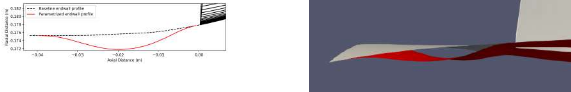
Figure 3.2: Parameterization of the endwall in the hub upstream region. On the meridional plane (left) and a 3D view (right).
