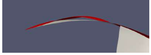
Figure 3.4: Parameterization of the endwall in the shroud upstream region. On the meridional plane (left) and a 3D view (right).
