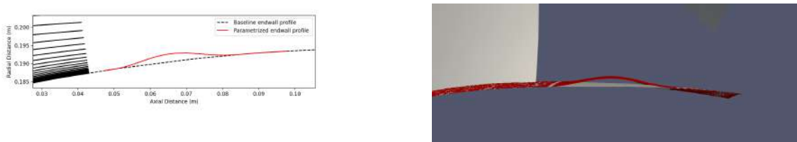
Figure 3.3: Parameterization of the endwall in the hub downstream region. On the meridional plane (left) and a 3D view (right).
