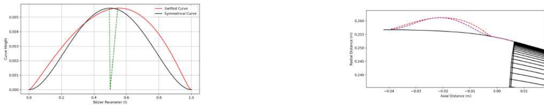
Figure 5.7: Comparison of the Bézier curve optimization (left) and the impact on the shroud meridional profile (right) in the upstream region of the shroud.
